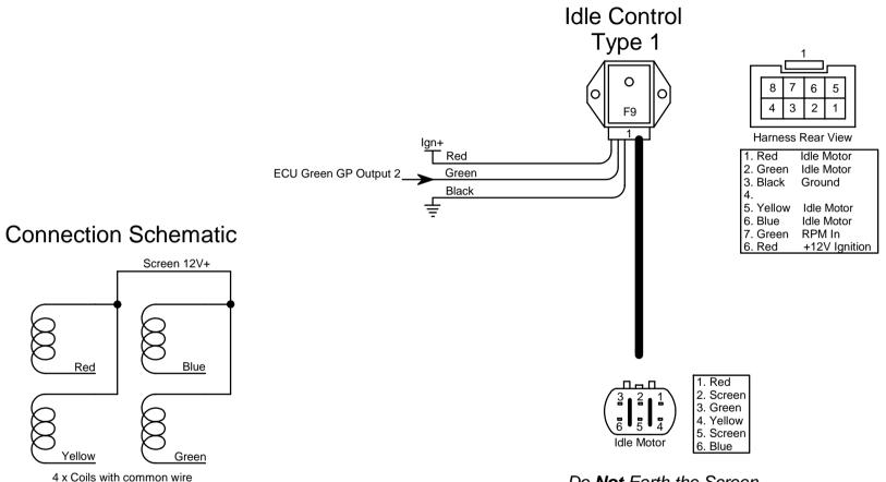
Do **Not u**se this idle control if coil resistance is less than 20 ohm!!!
